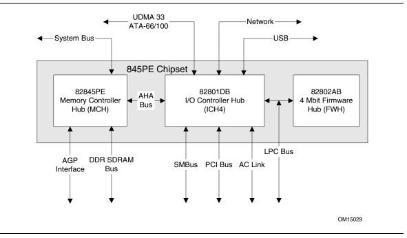
Figure 3. Intel 845PE Chipset Block Diagram
