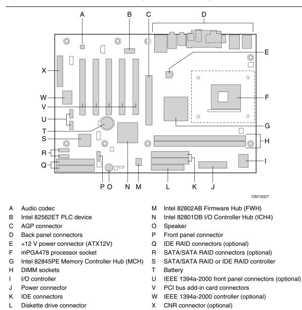
Figure 1 shows the location of the major components on the Desktop Board D845PEBT2.
