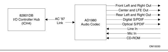
Figure 5. 6-Channel Audio Subsystem Block Diagram
