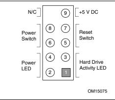
Figure 16. Front Panel Connector Pins
