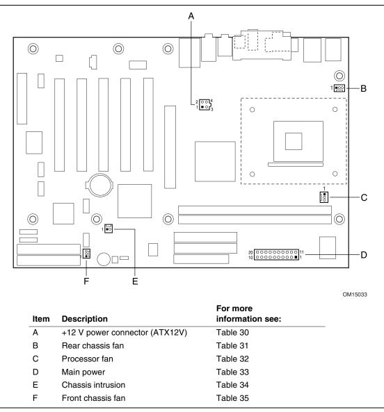
Figure 13. Power and Hardware Control Connectors
