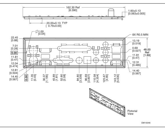
Figure 20. I/O Shield Dimensions for Boards with a 6-Channel Audio Subsystem and IEEE1394a-2000 Connector
