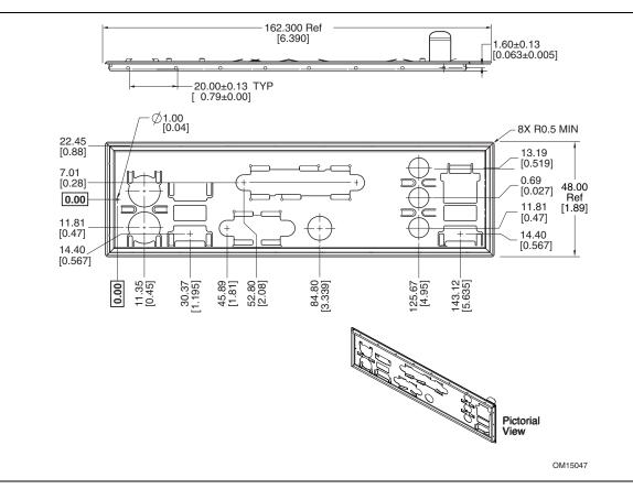
Figure 22. I/O Shield Dimensions for Boards with a 2-Channel Audio Subsystem
