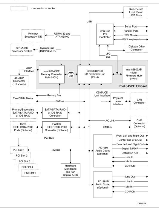
Figure 2. Block Diagram
