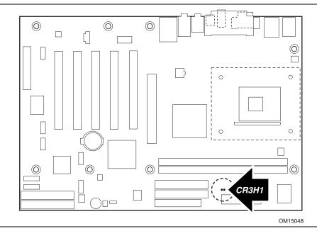
Figure 10. Location of the Standby Power Indicator LED
