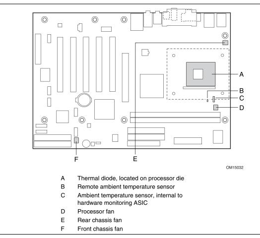
Figure 9. Thermal Monitoring
