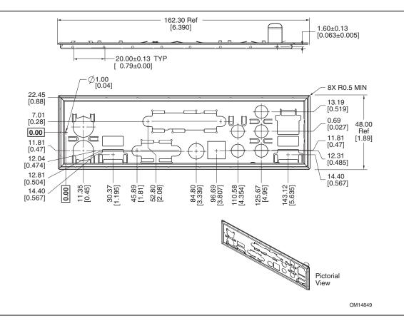
Figure 21. I/O Shield Dimensions for Boards with a 6-Channel Audio Subsystem and Without IEEE 1394a-2000 Connector
