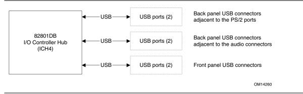
Figure 4. USB Port Configuration
