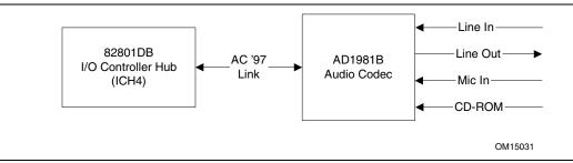
Figure 6. 2-Channel Audio Subsystem Block Diagram
