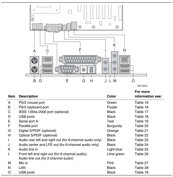
Figure 11. Back Panel Connectors
